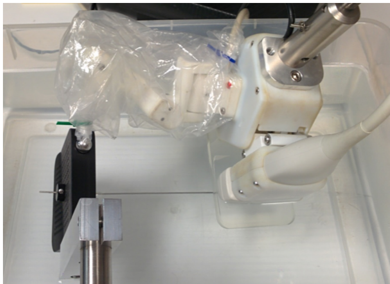
Figure 2.6: Experimental set-up for needle insertion through a tracked template. A collar affixed to the needle allows for a known insertion depth into a bath of isopropyl alcohol and water. Comparison of needle position in tracking and imaging quantifies tracking accuracy. Tracking arm has been bagged to prevent damage if immersed.
